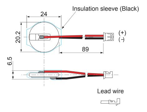
Contact: W125-0041-000 Housing: W125-0241-000 Wire: UL1007 AWG28
